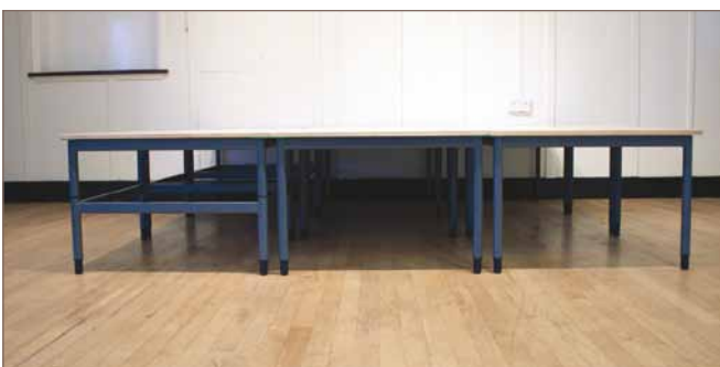
Examples show that moving frames from the front row to the back, creates stepped staging from flat.
